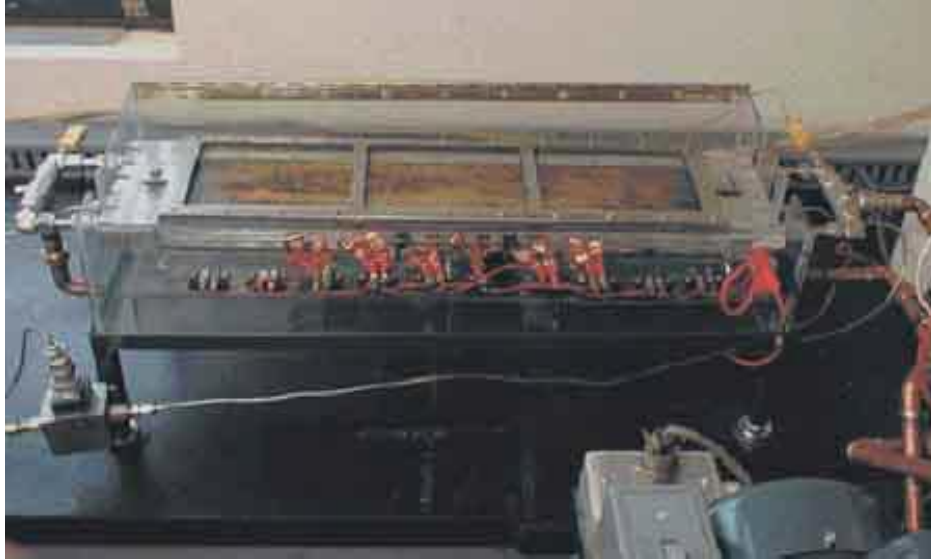
Figure 2.13: Water flow control and thin film assembly system housing for temperature cycling used by Ikura et al [17].
