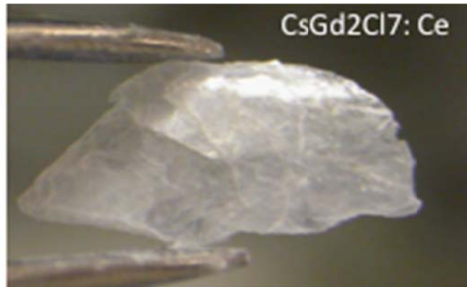
Figure 3.6 Crystals of \text{CsGd}_2\text{Cl}_7:\text{Ce}^{3+} synthesized in a vacuum sealed ampoule; the above sample is approximately 5 mm long in the horizontal axis.
