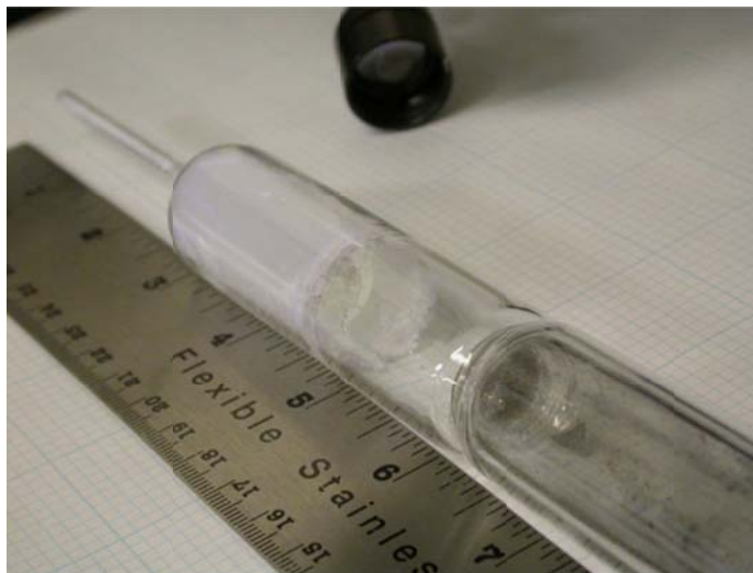
Figure 2.4 Crystal growth ampoule with a melt filtration tube
