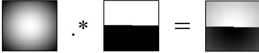
Figure 3.2: Building a polarized Gaussian kernel by multiplying a Gaussian kernel with a binary mask, where “ \cdot ” represents the element-wise multiplication.
