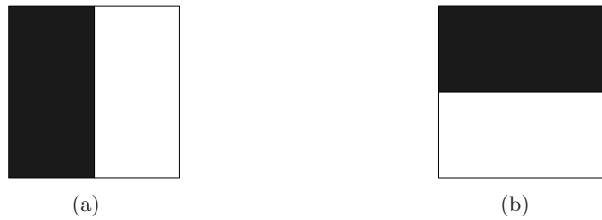
Figure 2.11: Haar wavelet templates to compute the responses along horizontal (a) and vertical (b) directions.
