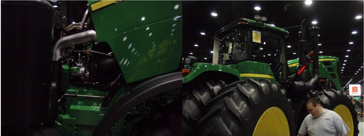
Figure F.1: The cEGR exhaust system on several JD tractors on display at the 2011 National Farm Machinery Show in Louisville, KY. On the left, exhaust, laden with PM is funneled from the engine into a DOC. On the right, the much larger exhaust system needed for Tier IV engines to accommodate the DOC and DPF (pictures taken by author).
