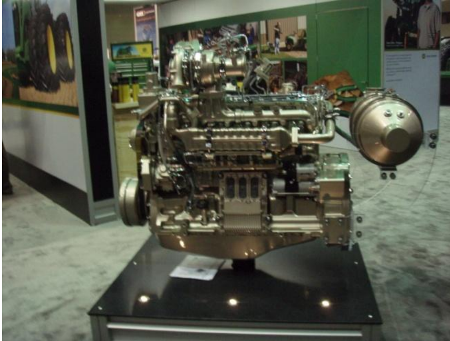
Figure 5.40: Deere's prototype cEGR engine for farm tractors on display at the 2010 Ag Connect Expo in Orlando, FL (picture taken by author).
