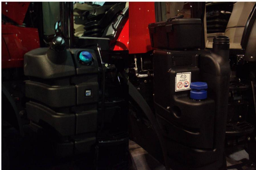
Figure F.3: SCR fuel tanks (left to right) of a Massey-Ferguson and Case IH tractor. The blue cap is on the tank for DEF and has a smaller filling neck to prevent introduction of diesel fuel (pictures taken by author).
