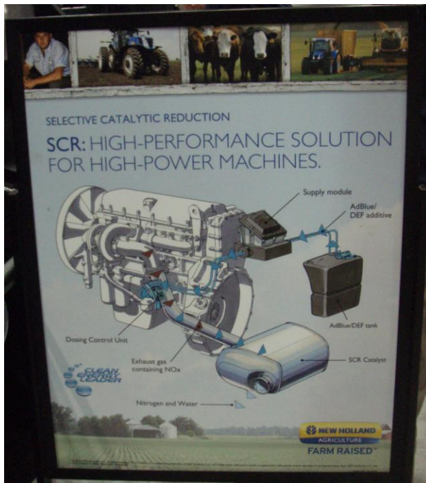
Figure 5.39: A sign in New Holland's display area explaining SCR at the 2011 National Farm Machinery Show in Louisville, KY (picture taken by author).
