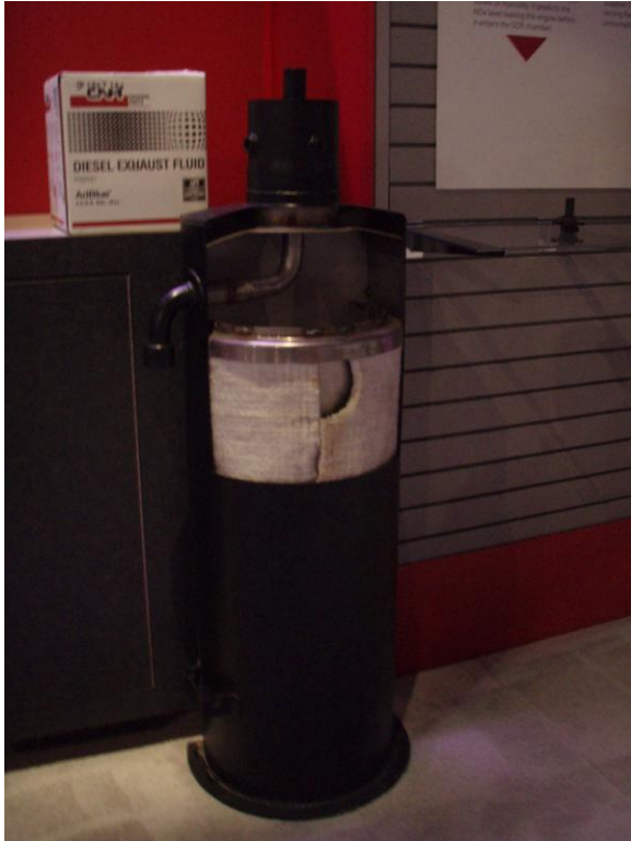
Figure F.2: A cutaway view of the exhaust muffler for a Case IH SCR engine. At the top is the catalytic chamber where DEF is introduced and at the bottom is the DPF (picture taken by author).
