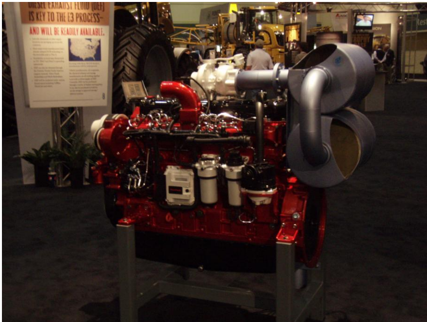
Figure 2.2: An AGCO E 3 Sisu low emission diesel engine, employing SCR technology, on display at Ag Connect Expo in Orlando, FL in 2010 (picture taken by author).
