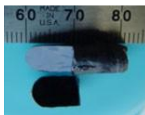
Figure 2.11 Single crystal of \text{Sr}_2\text{RuO}_4 grown by floating zone technique in ORNL
