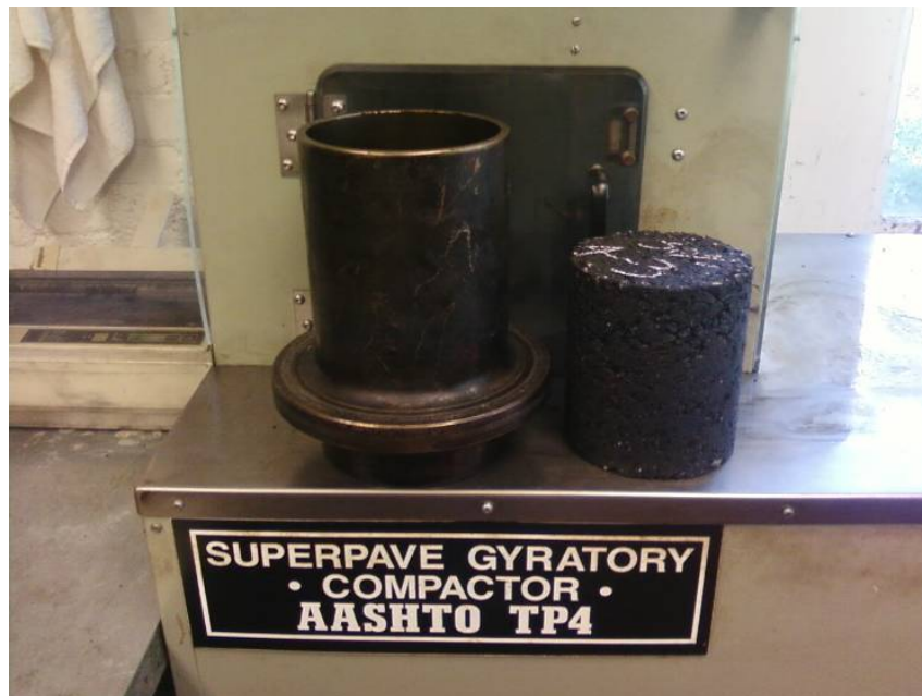
Figure 4.6 Laboratory SGC compaction test
