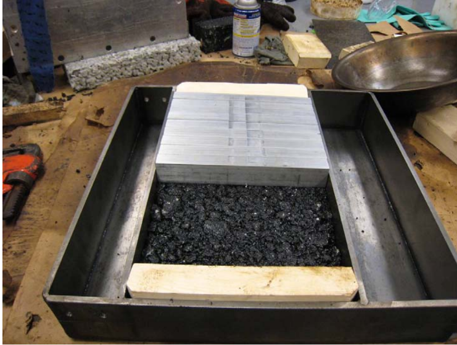
Figure 6.4 Asphalt mixture compacted with APA linear kneading compactor
