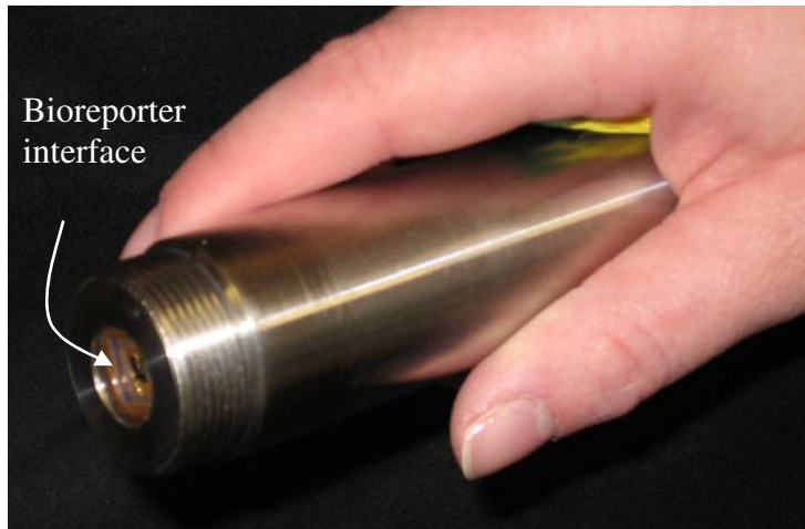
Figure 2. Example of a CMOS microluminometer transducer in a hand-held biosensor format.
