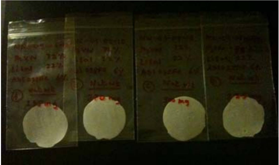
Figure 19. Li-Sal/P2VN Film Detectors
