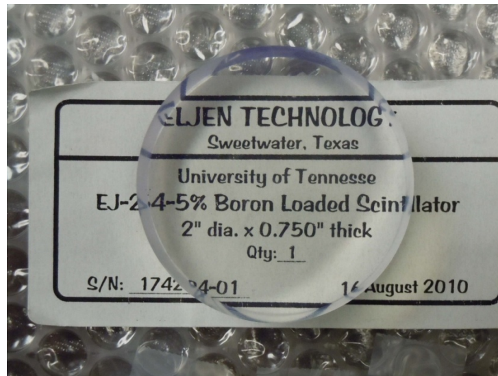
Figure 29. Eljen 10 B-Based Plastic Scintillation Detector
