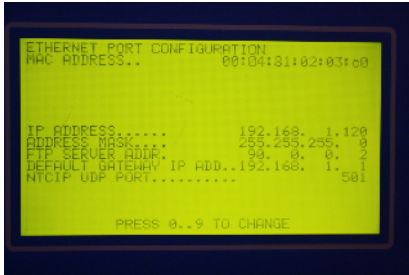
Figure 11 - ASC/3 Ethernet port configuration
