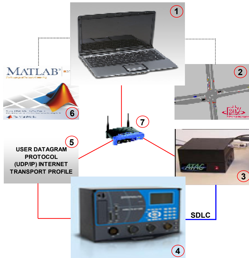
Figure 1 - System architecture for a hardware-in-the-loop simulation (1-Computer, 2-Traffic Simulator, 3-Controller Interface Device, 4-Traffic Signal Controller, 5-Communication Protocol, 6-Algorithm Software, 7-Ethernet Connection Provider)
