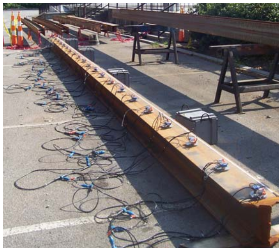
Figure 7.1. Simply supported test beam (HP12x53) instrumented with geophones
