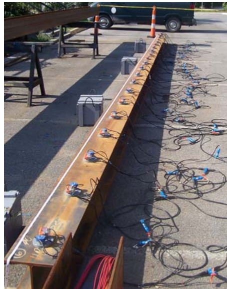
Figure 3.1. Simply supported test beam (HP12x53) instrumented with geophones
