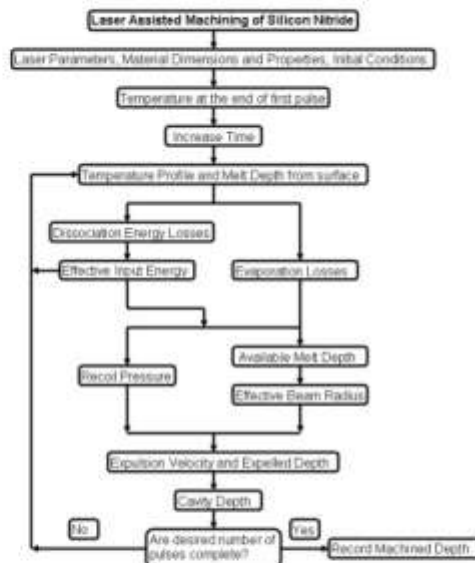
Fig. 3. Stepwise procedure for machined cavity depth prediction.
