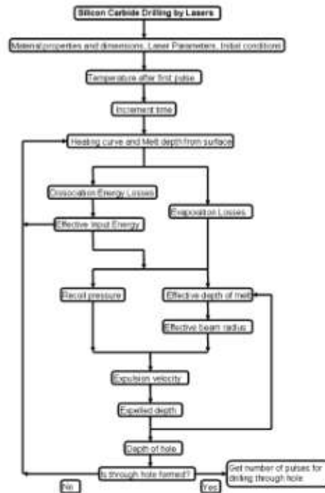
Fig. 7 Flowchart showing procedure for prediction of drilled depth
