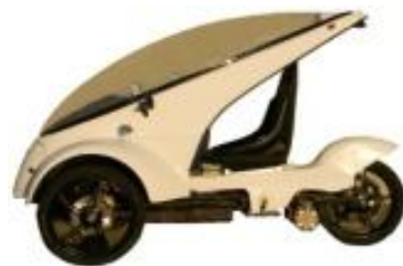
Figure 1. The commercially available BugE ® frame and chassis kit.
