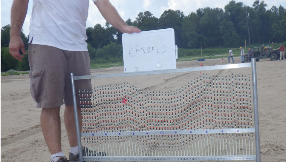
Figure 1: Example picture of rut profile and meter, from which pin readings were taken. Test indicated is CM8FLD, which corresponds to coarse grain, multi-pass number eight, fast speed, low pressure, driver side.
