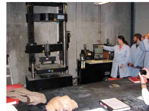
Dr. Stephanie TerMaath, pointing at the computer screen, and students test a composite beam from the Strongwell Corporation in the Department of Civil and Environmental Engineering lab.
