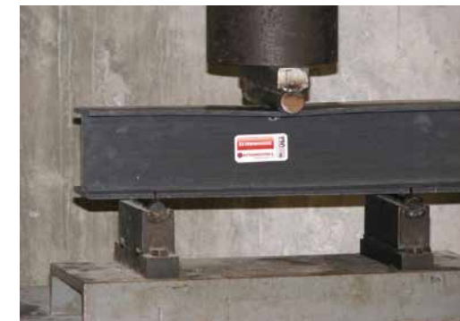
A composite beam from the Strongwell Corporation is put under pressure in a beam-bending test in the Department of Civil and Environmental Engineering lab.
