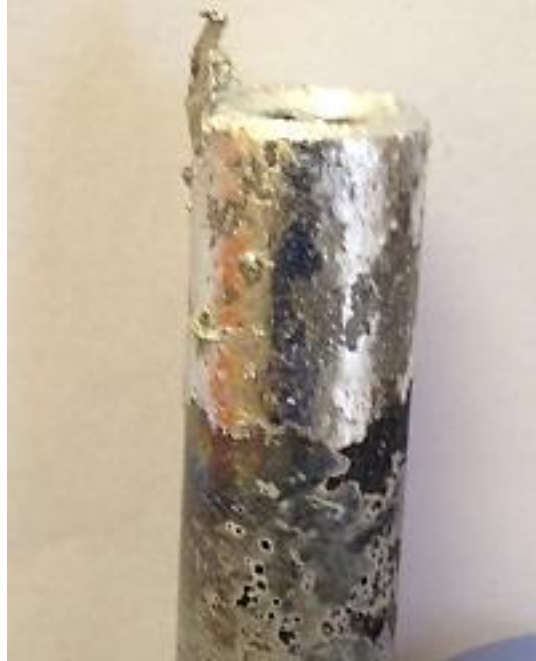
Figure 10 Sample using Ultra Flux II and dipped at 473 °C
