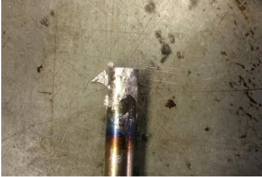
Figure 11 Alloy coating on zircalloy with acid preparation and alloy temperature of 650 °C
