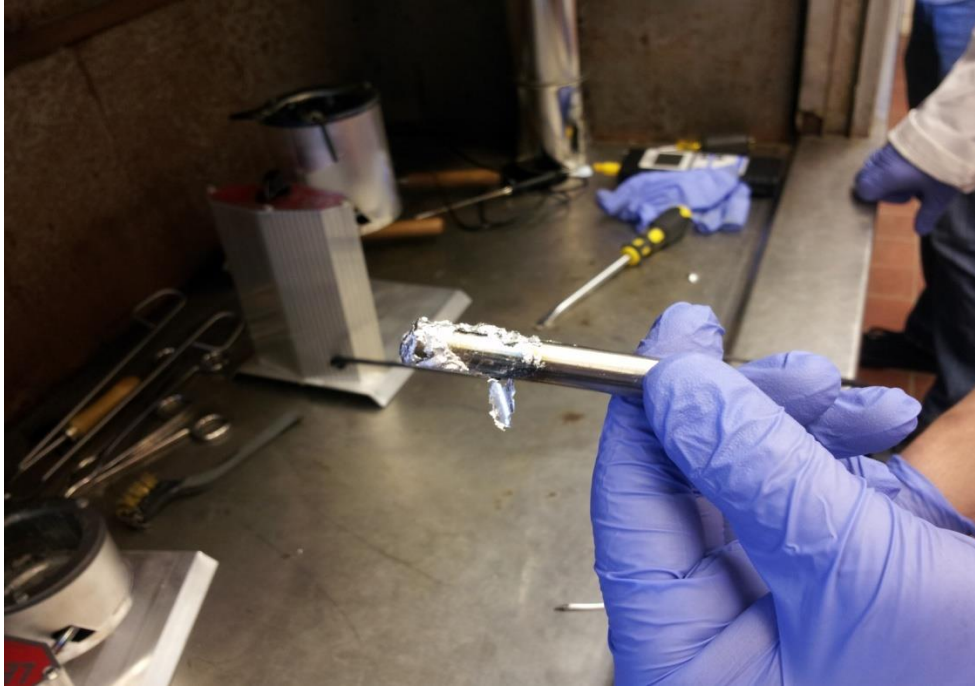
Figure 8 Sample without surface preparation at 350 °C after alloy has been partially removed by force
