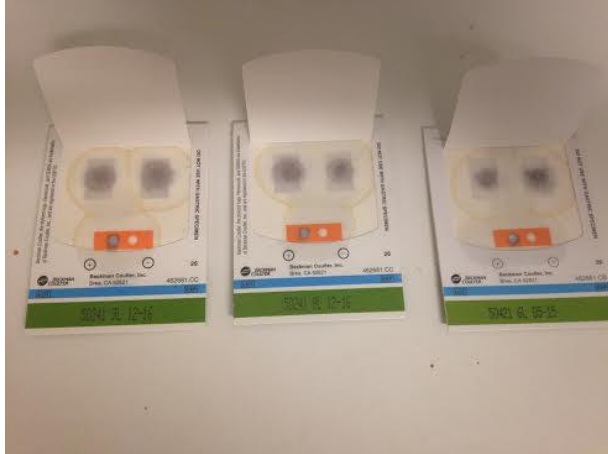
Figure 16: Visible color change, indicating positive heme detection, following the 2ml test
