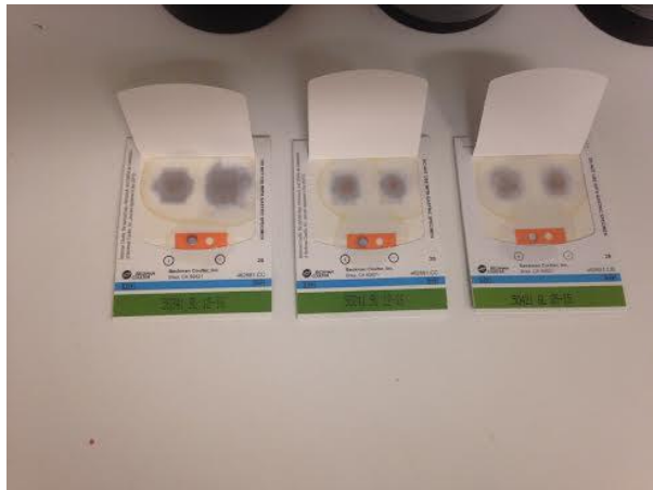
Figure 17: More notable color change, indicating positive heme detection, following the 4ml test
