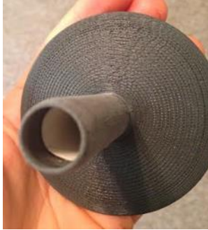
Figure 10: Gum guaiac test paper lining inside of body cylinder
