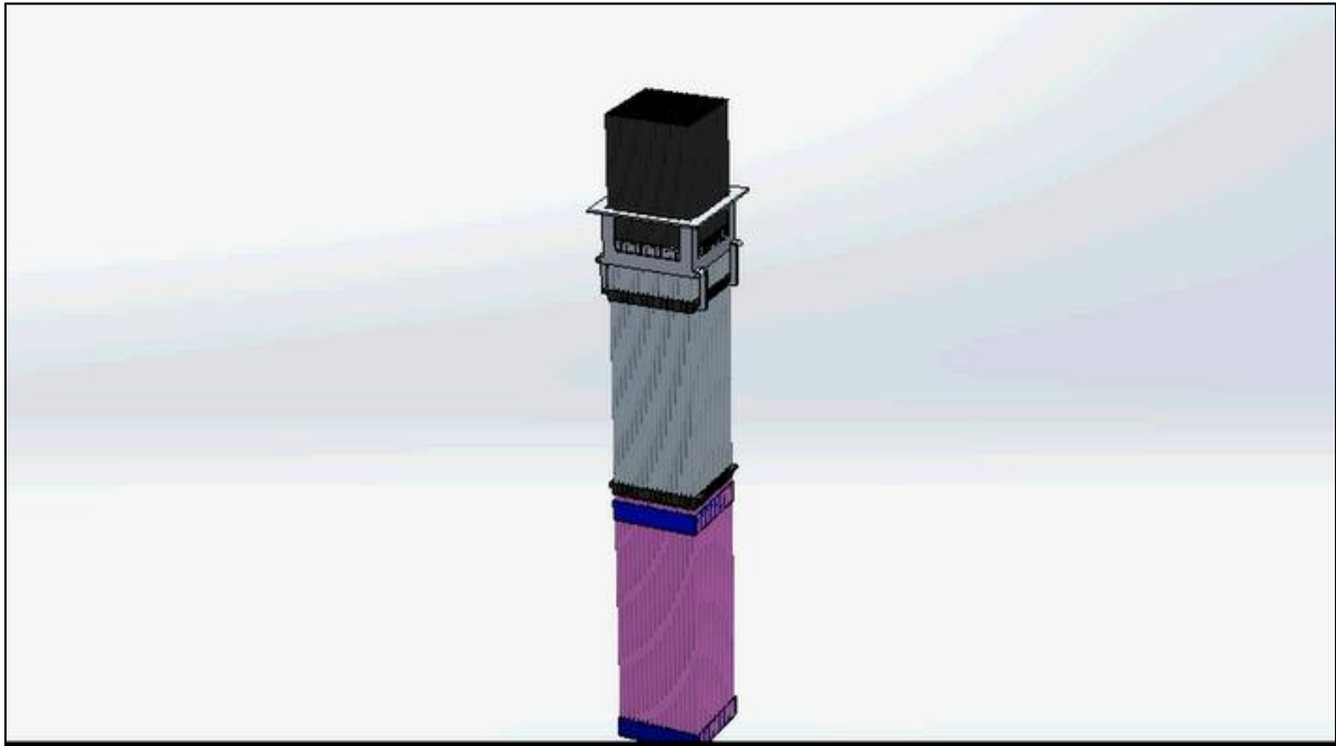
Figure 13: The lifting device placing the fuel assembly above the stainless steel tube assembly, with the driving rods preparing for the fuel rods to be pushed into the tubes
