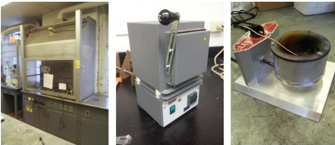
Figure 2: Chemical hood, furnace, and melting pot used in our experiments (L to R)
