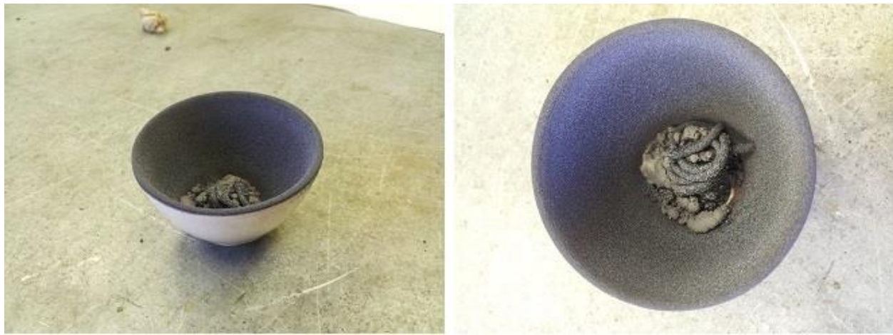
Figure 3: Ceramic crucible containing oxidized cadmium and copper
