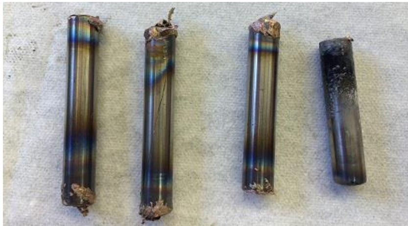
Figure 4: Zircaloy tubing samples after Ag45 dip application
