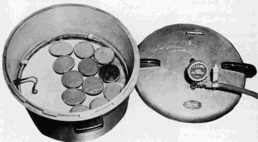
Figure 3. Saturated soil samples on a ceramic pressure plate for the 1/3 atmosphere tension determination.
