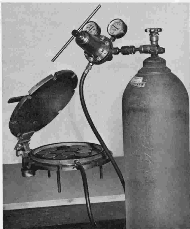
Figure 4. Saturat- ed soil samples on a pressure membrane for the 2, 5, 9 or 15 atmosphere ten- sion determina- tion.
