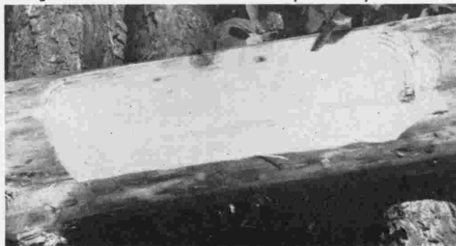
Figure 4. Two entrance holes of pine sawyer larvae are visible in a strip about 1 foot long, on the upper side of a bug-peeled post that was crib-piled for 150 days in the bottom layer. The insects were not very active in the warmer and drier upper side of the post. (TVA photo)
