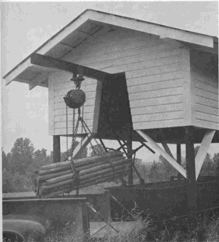
Figure 6. Posts were chained together before immersion in the sheltered treating vat.
