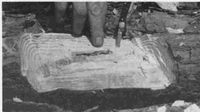
Figure 3. These large-diameter posts were dead-piled for 90 days and exposed to insect action. Pine sawyer larvae have attacked the posts. (TVA photo)
