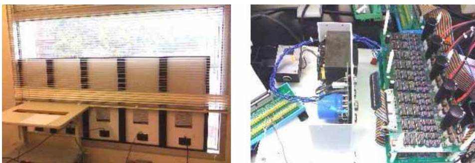
Figure 3. Experimental setups. (a) PV Module comprised of five solar panels. (b) 11-level (5 H-bridges) cascaded multilevel converter.
