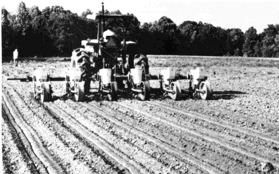
Figure 1. Six-row planter mounted on a rigid tool bar and used on conventional and bedded plots in 1974 and 1975.
