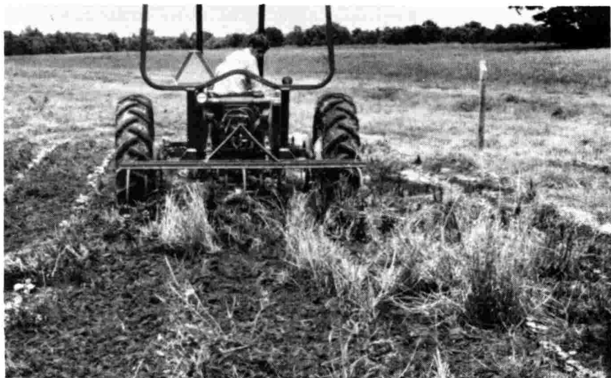
Figure 3. Killed sod and grass collected on cultivator sweeps during first cultivation of no till plots in 1974.
