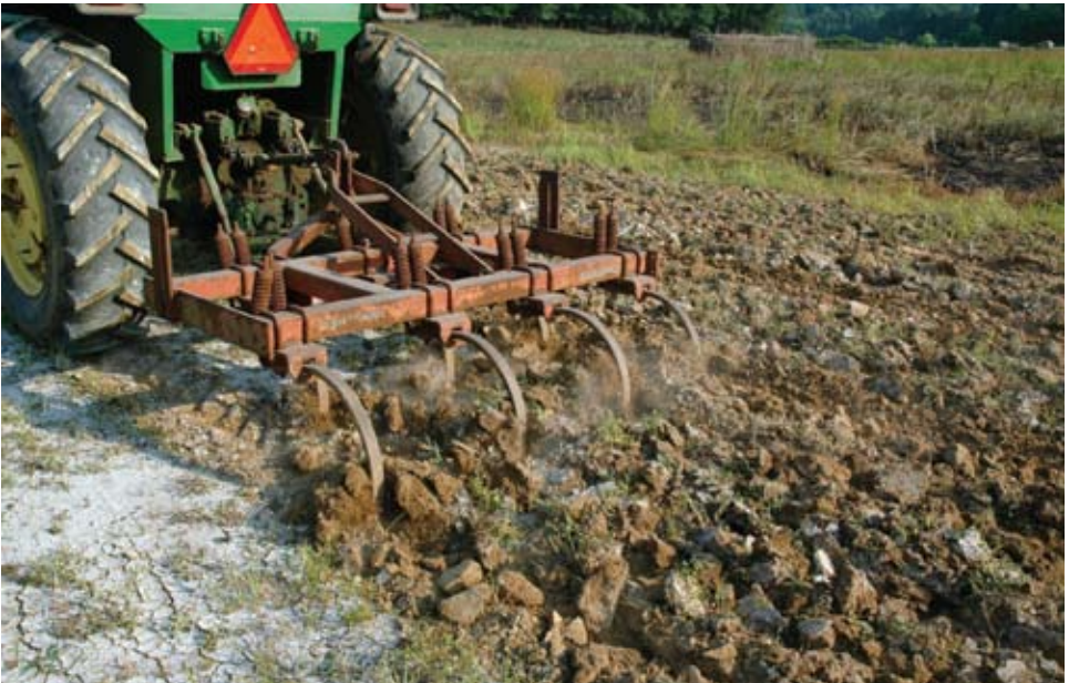
Fig. 4.7 A chisel plow with shanks 16–20 inches long does a great job incorporating lime and breaking hardpans created after many years of disking and shallow plowing.
