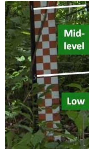
Figure 2. Checkered profile board used for measuring percent vertical cover of vegetation in 0 – 20 inches (low) and 20 – 40 inches (mid-level) height strata. There are 30 2-by-2-inch boxes per stratum.
