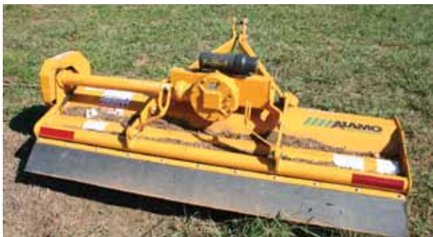
The flail mower finely chops and uniformly distributes plant residue on the soil surface.
