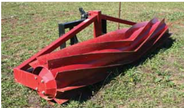
The roller crimper, with angle iron blades, crimps the stems and lays the intact plant uniformly on the ground.
