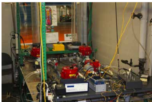
Figure 2.1: Experimental flow loop used for experiments and equipped with MOVs, flow and pressure sensors, along with a full data acquisition system interfaced with a PC
