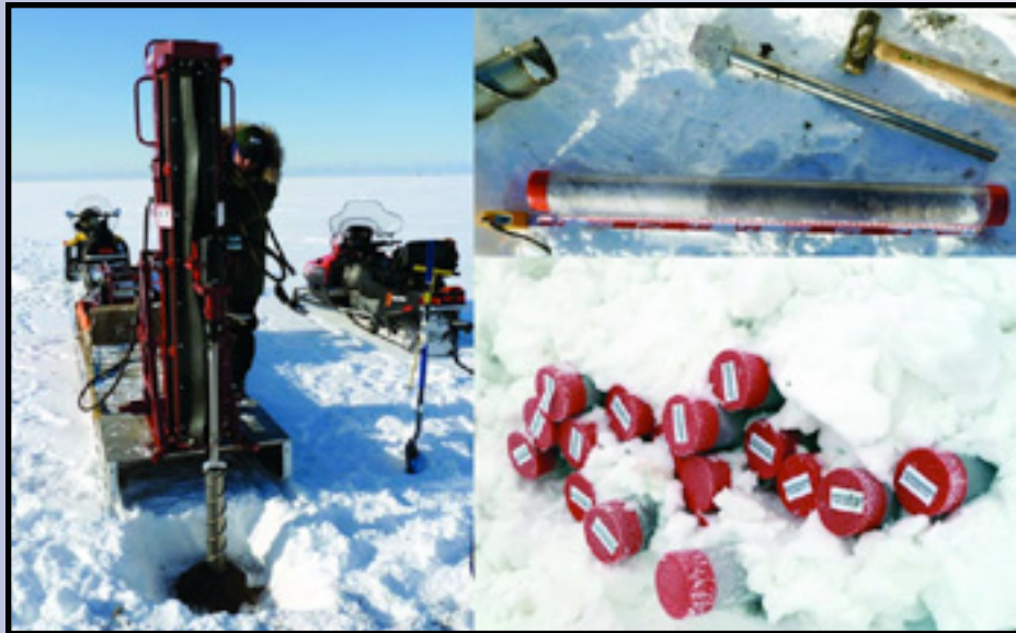
The ORNL NGEE-Arctic team used a sled-mounted hydraulic drill to remove samples of permafrost tundra in Barrow, Alaska for biogeochemical analysis of microbial activity and carbon transformation (left). Core samples included significant amounts of ground ice and organic matter that has been preserved, frozen for hundreds or thousands of years (top, right). The cores were stored frozen in snowbanks to prevent thawing before shipment to Oak Ridge (bottom, right). Image Credit: David Graham, ORNL.
