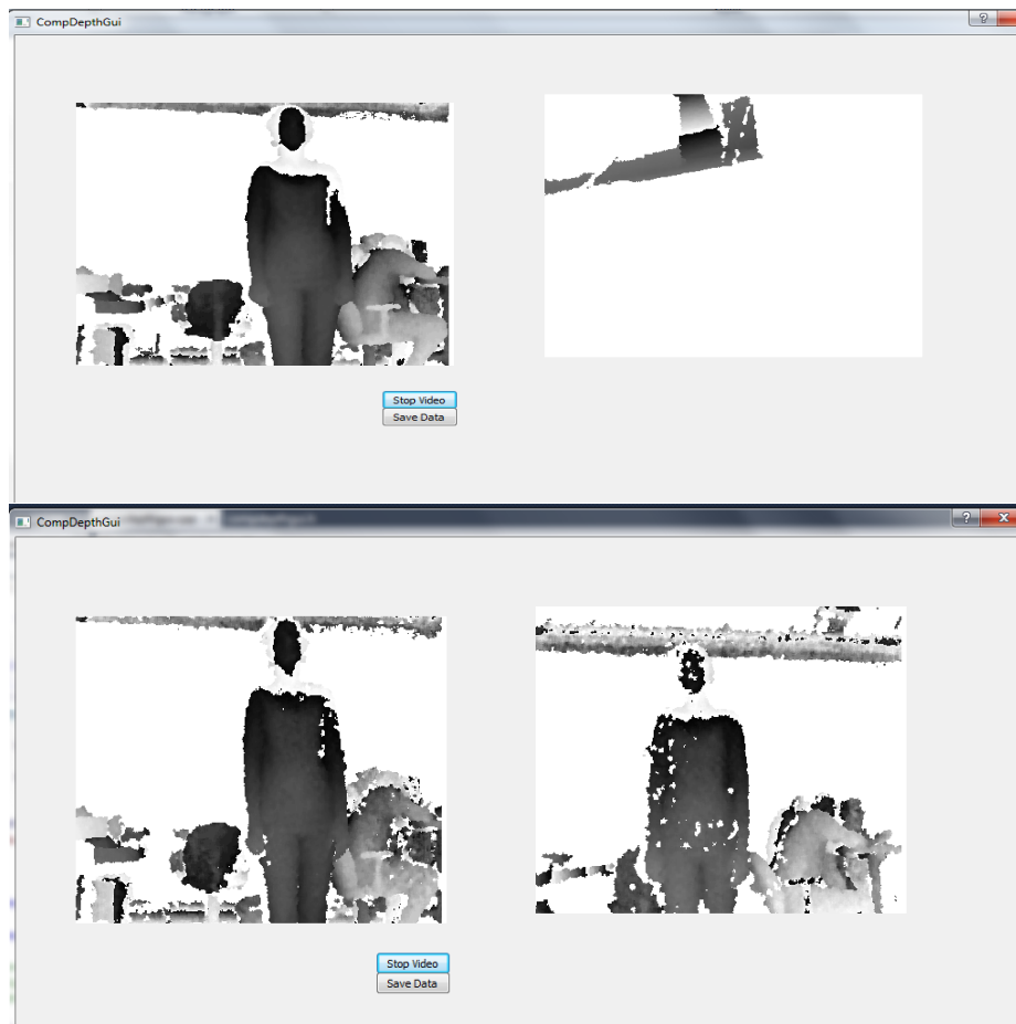
Figure 10. Above shows a depth image using a single Kinect. Below is the difference when two are used. Note the surprising lack of excess speckling in the left picture, but marked speckling on the right.
