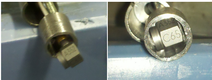
Figure 14: Accelerometer Placed in Casing Prior to Testing
