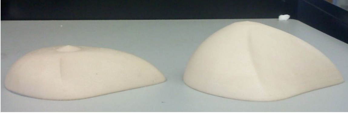
Figure 9: Side-by-side view of the two iterations of the computer-modeled breast printed for a phantom mold
