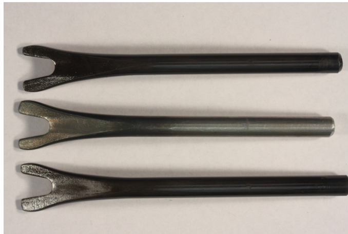
Figure 5: Solution 3 samples have a thin but consistent layer
