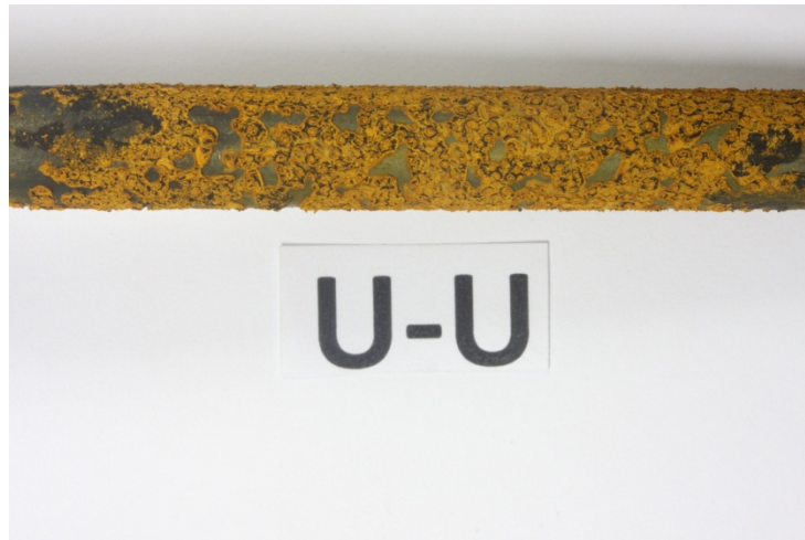
Figure 15: U-U sample has significant rust formation.
