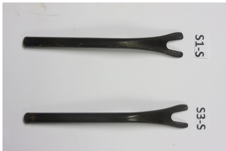
Figure 13: S1-S sample shows many rust spots. S3-S sample has no rust formation on the head and shaft except the unexplained ring located near the bottom
