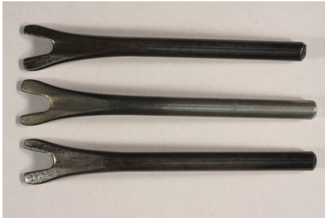
Figure 4: Samples coated using solution 2 resulted in an inconsistent layer
