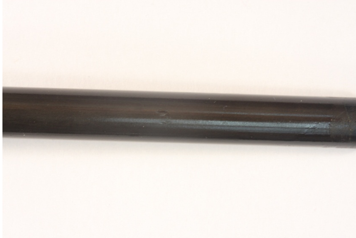
Figure 8: Solution 3, thin but consistent layer
