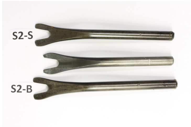
Figure 10: Solution 2 samples showed no rust except on the bottom of S2-B
