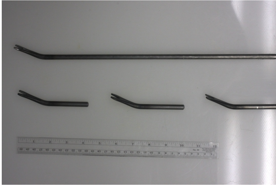
Figure 2: Macrograph showing the two sample sizes which will be used for creating a brown surface finish.
