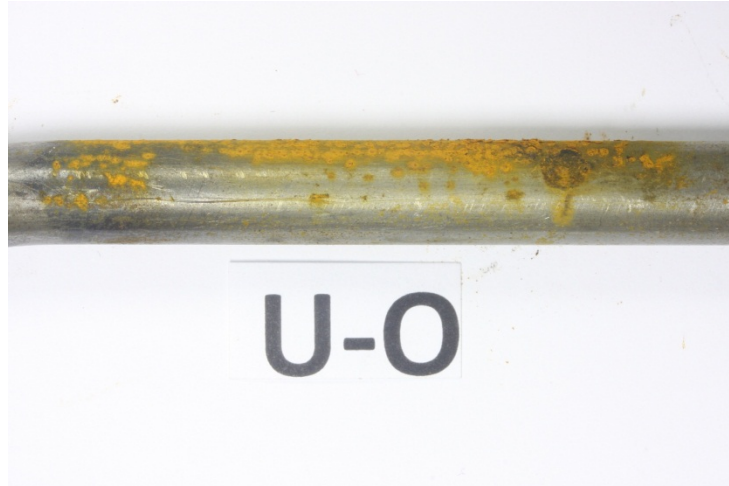
Figure 14: U-O sample shows some rust prevention from the tung oil.
