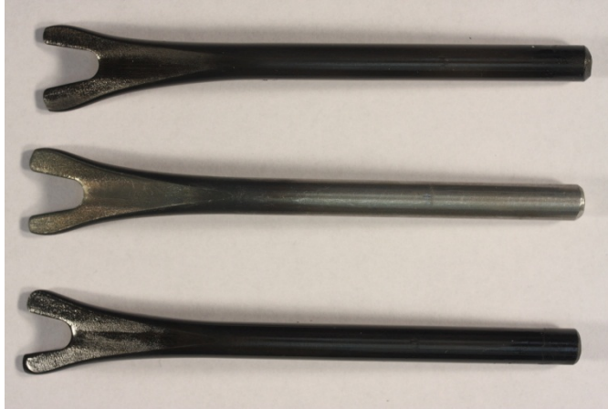
Figure 3: Samples coated with solution 1 have a thick consistent layer.
