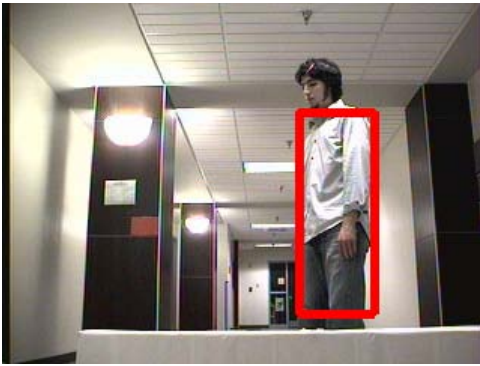
Fig. 4. After building a target model with the training image shown in Fig. 2, shown here is a single frame of kernel-based object tracking from the experimental recording on April 19, 2009. Correlation is 0.40964 between candidate color histogram derivative (a forward finite difference) with that of the target model. The camera frame size is 320 \times 240 pixels.
