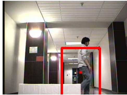
Fig. 3. After building a target model with the training image shown in Fig. 2, shown here is a single frame of kernel-based object tracking from the experimental recording on April 19, 2009. Note that the bright light in the upper-left corner of the image sometimes “distracted” the tracker for periods of several seconds when the target walked under it. The camera frame size is 320 \times 240 pixels.
