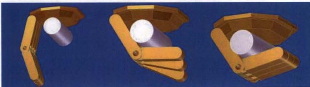
Figure 16. Stages of 0° wrap grasp
