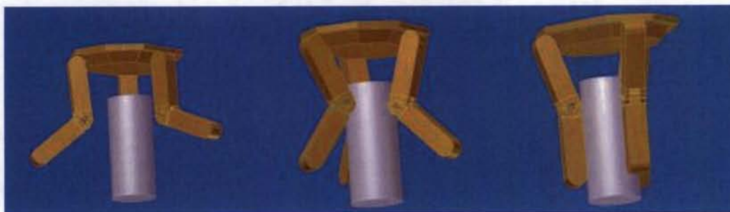
Figure 18. Stages of 120^\circ finger pad grasp
