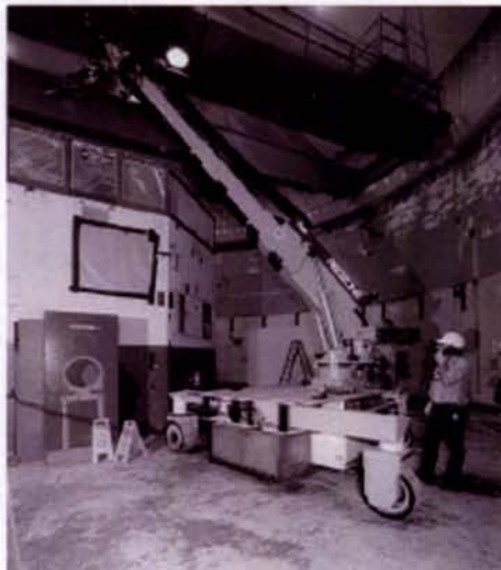
Figure 1. Rosie with jackhammer end-effector [8]
