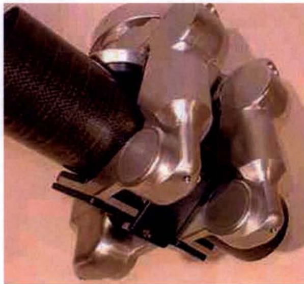
Figure 5. BarrettWraptor™ with pipe
