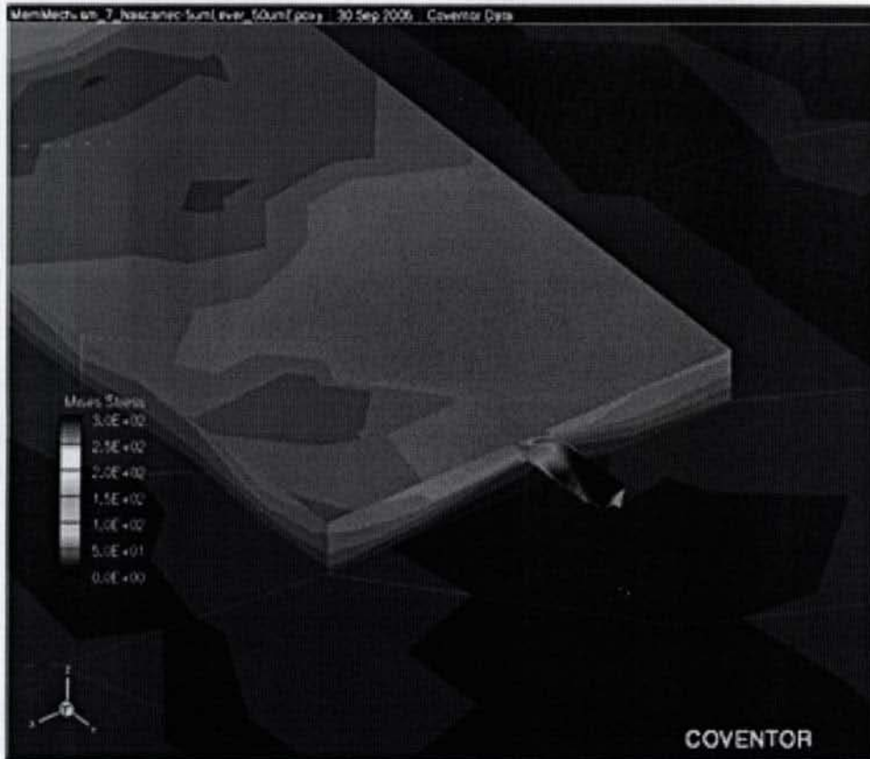
FIGURE 4: COVENTOR DEFLECTION ANALYSIS FOR A MICROCANTILEVER SUBJECTED TO LOADING.
