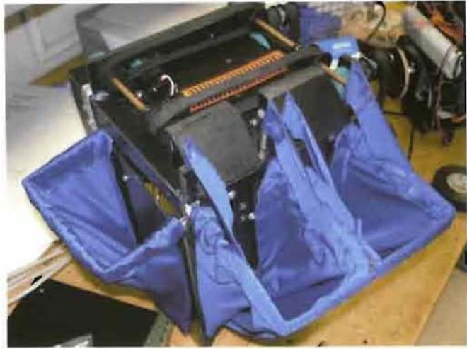
Figure 14: Storage Bins with Spandex
