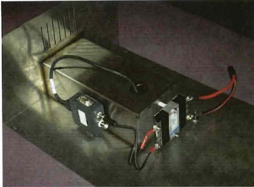
Figure 7: Lid showing power converter for camera and camera connection box.
