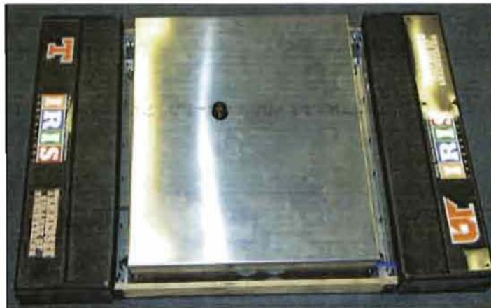
Figure 1: Original thermal brick in Safebot. (Image courtesy of Nikhil Naik)
