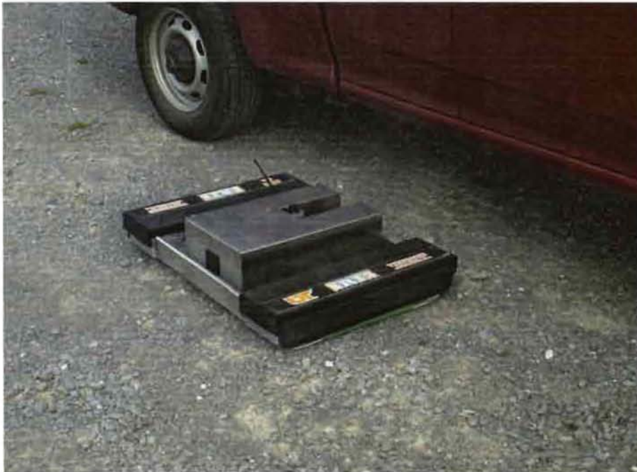
Figure 2: New brick in Safobot, ready to inspect underneath a vehicle.
