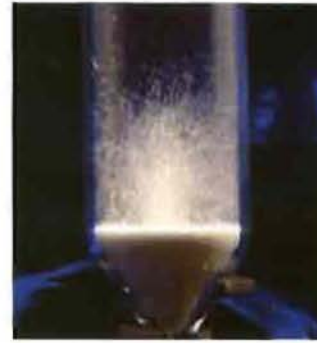
Figure 16: Fluidized bed reactor (~30 LPM airflow)
