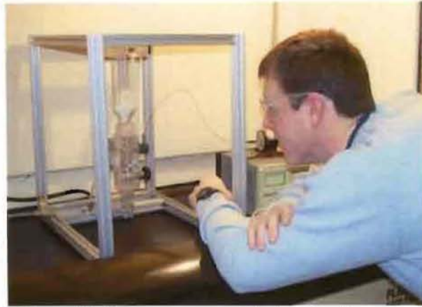
Figure 12: Pressure sensor collecting data from reactor
