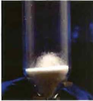
Figure 15: Fluidized bed reactor (~20 LPM airflow)
