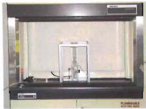
Figure 5: Fluidized Bed Reactor, frame, and modular pieces in hood
