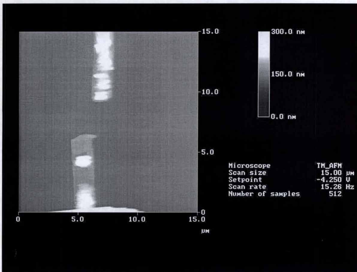
Figure 8: Condition of device #6 after multiple deposition and dissolution of Ni (top electrode negative, bottom electrode positive)
