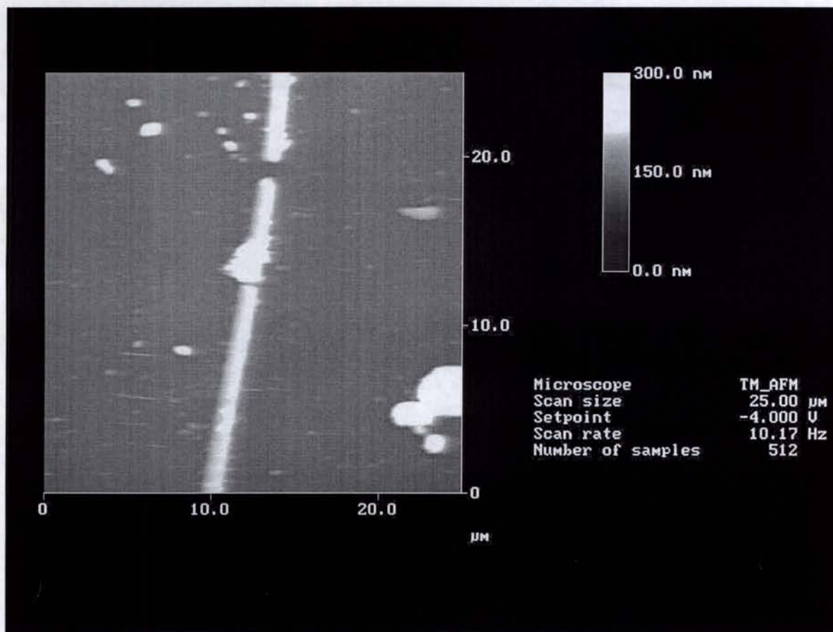
Figure 6: Pre-experiment condition of device #4
