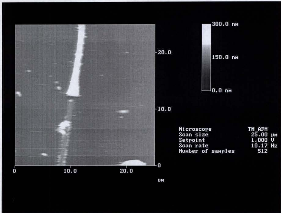
Figure 7: Condition of device #4 after multiple deposition and dissolution of Ni (top electrode negative, bottom electrode ground)
