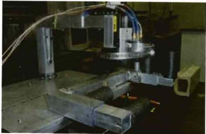
Figure 7: Finished device, emphasizing the arm fixture and shaker support
