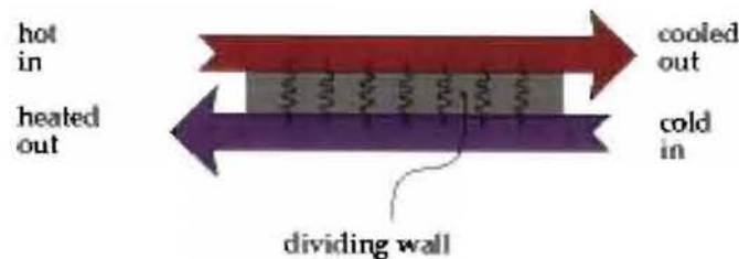
Figure 14: Heat exchanger in a recuperator
