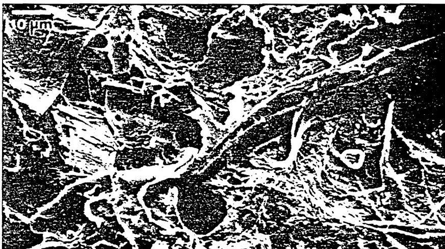
7. SEM of hot-pressed PHB latex coated paper after 12 days immersion in simulated activated sludge
