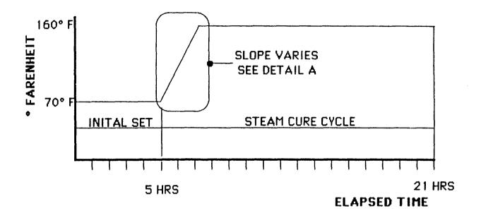
FIGURE 1: TYPICAL THERMAL EXPOSURE OF STEAM CURED SPECIMENS
