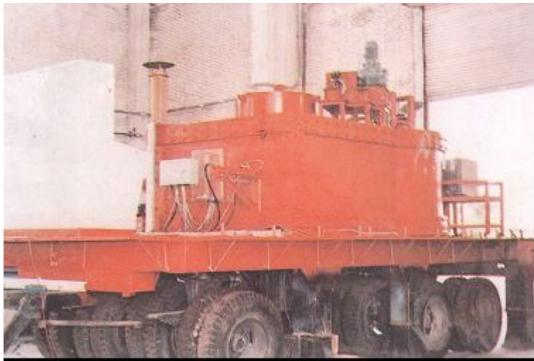
Figure 2.1: A large mobile irradiator (Beijing Institute of Nuclear Engineering) containing 250,000-curies of cesium-137
