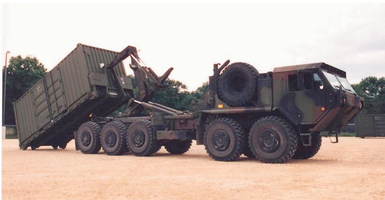
Figure 4.4.2: A PLS with its CHU extended to unload an ISO container 15
