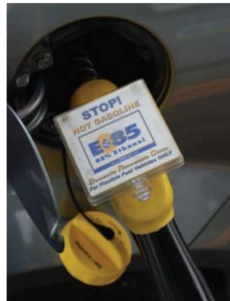
E-85 dispensers are clearly labeled. You can see the yellow gas cap indicating a flex fuel vehicle in the background. Credit: Sam Jackson, University of Tennessee
