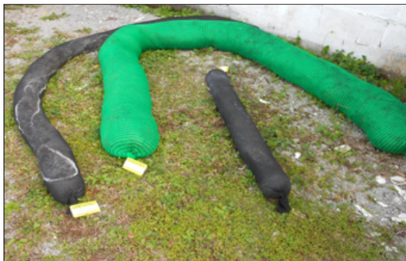
Figure 3. Bacteria media filter socks and an installation site along Vista Drive in Horry County.
