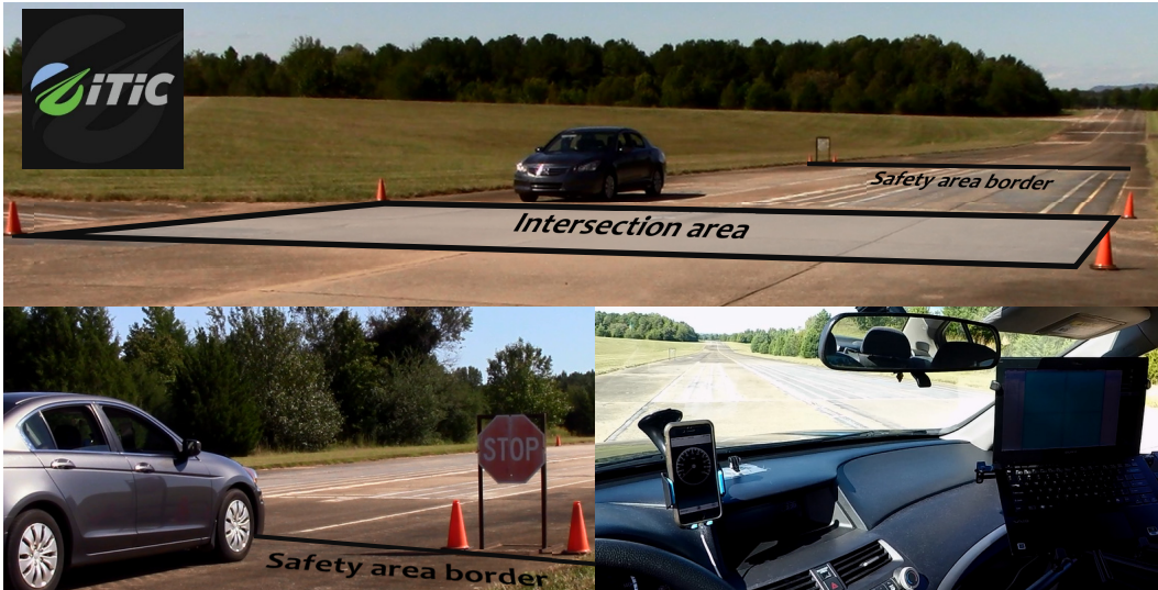
Figure 9.6: The vehicle-in-the-loop test area at International Transportation Innovation Center (ITIC).
