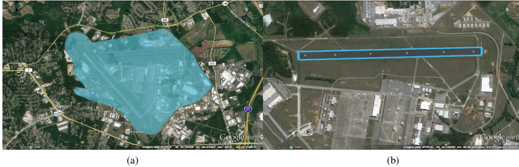
Figure 9.5: Google satellite view of (a) International Transportation Innovation Center (ITIC) test site (b) the 5,500 x 300-foot asphalt straightaway used to execute the vehicle-in-the-loop tests.
