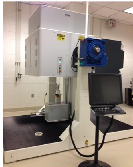
Figure 8: Clemson Universities MILabs Vector4 Pre-clinical CT machine with vertical imaging bed orientation.
