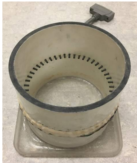
Appendix 3.4 : ERT array testing column.
