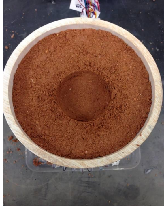
Appendix 3.5 : ERT array testing columns. Column on left shows wetted soil with air void target design, where the column shown on the right has wetted soil with a dryer more resistive soil core target. Similarly, an air void is created in the center of a NaCl solution sample by placing an empty glass beaker in the center of the imaging field.
