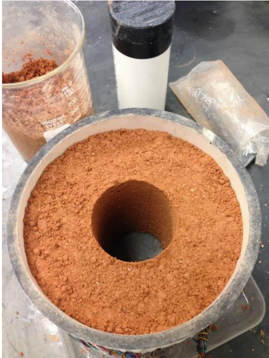
Appendix 3.5 : ERT array testing columns. Column on left shows wetted soil with air void target design, where the column shown on the right has wetted soil with a dryer more resistive soil core target. Similarly, an air void is created in the center of a NaCl solution sample by placing an empty glass beaker in the center of the imaging field.
