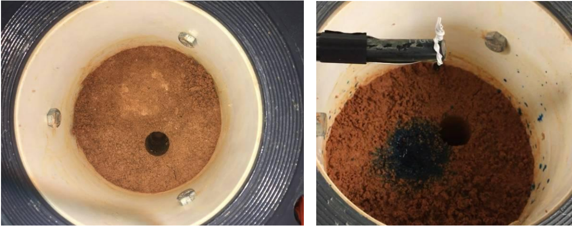
Appendix 5.7: Photo on left shows the offset orientation of engineered macropore. Photo on right shows drip location of irrigation indicated by blue tracer dye.
