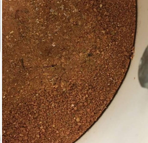
Appendix 5.6 : Contact area between soil matrix and column wall at the upper soil boundary. A small gap is seen to have developed as soil shrinks from drying.
