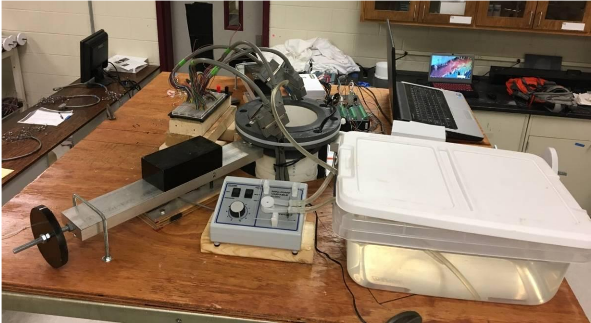
Appendix 5.4 : Photo of setup of steady low flow infiltration experiment. Peristaltic pump feeds influent from reservoir into the columns upper surface (Appx. 4.5).
