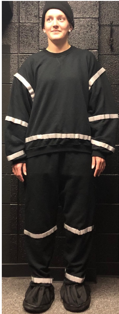
Figure 1. Retroreflective strips were placed on the test pedestrian's major joints. In the biomotion configuration, the pedestrians walked in place, while the pedestrian stood still in the standing condition. In all conditions the pedestrian was positioned on a sidewalk immediately to the right of the test vehicle's lane of travel, facing the oncoming test vehicle.
