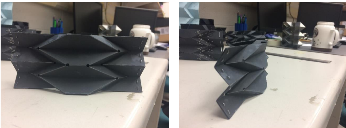
Figure 18: Optimized TMP Bellows Design Manufactured from Polypropylene
