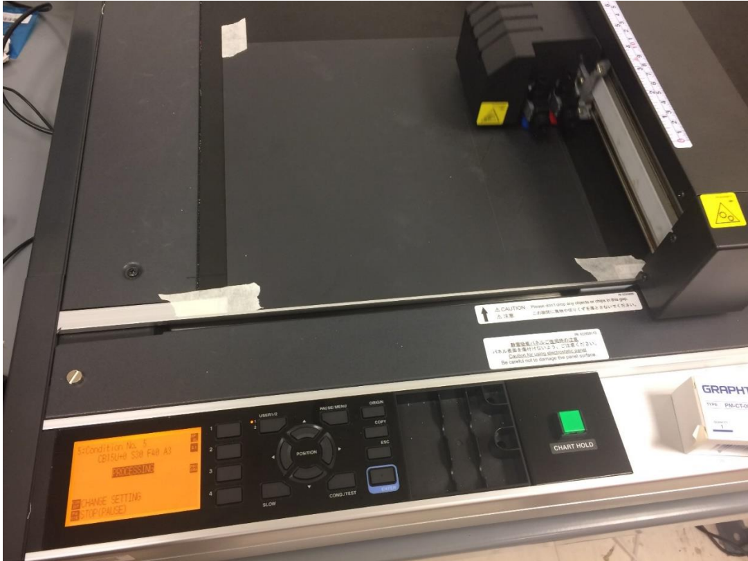
Figure 14: The FCX4000 Cutter In progress Cutting the Grooves and Stress Reliefs for one of the Necessary Sheets for the TMP Bellows
