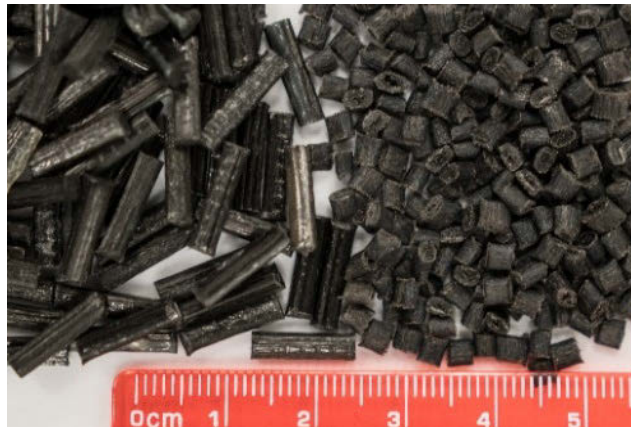
Figure 3.1 Short fiber and long fiber reinforced thermoplastic pellets.
