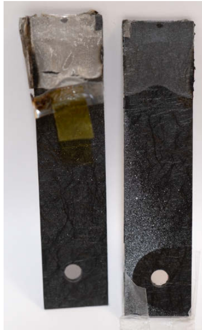
Figure 7.10 Interfacial failure during Double cantilever beam test.
