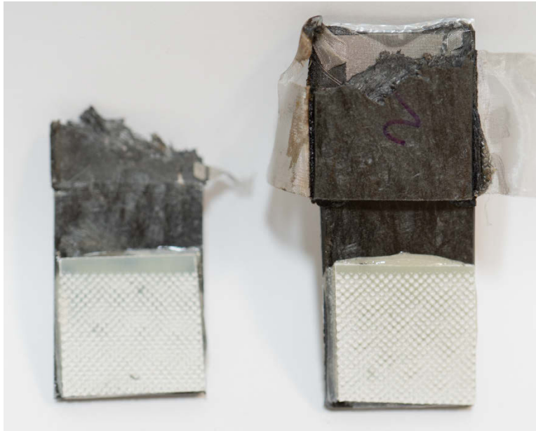
Figure 7.7 LFT coupons after failures.
