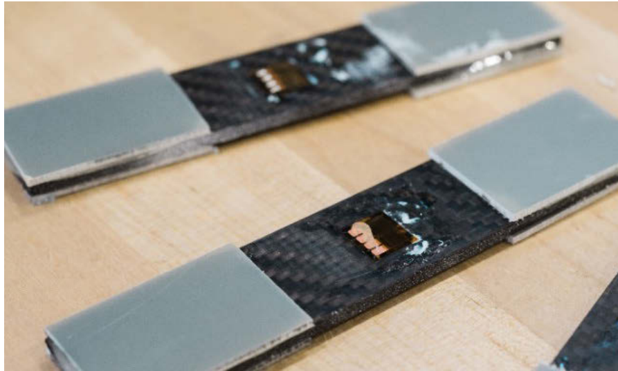
Figure 3.6 Woven test coupons with bonded strain gauges and glass fiber tabs.
