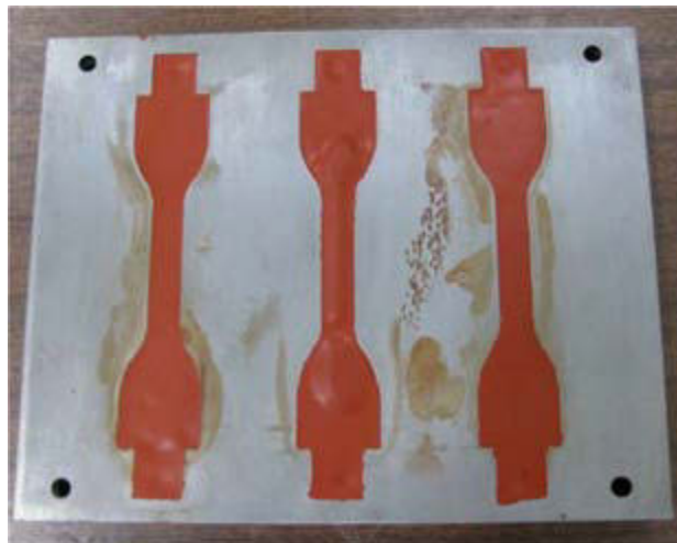
Figure 2.10 Tensile samples for bulk characterization of adhesive. (image source 89 )
