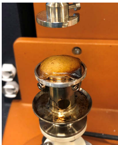
Figure 6.8 Visual color change (degradation) in pure PA66 at ~290°C.
